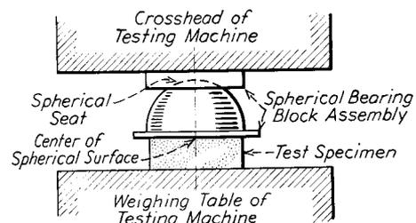
FIG. 4 Spherical Bearing Block for Compressive Strength Test
