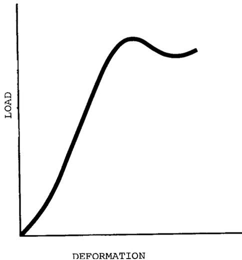
FIG. 1 Procedure A—Straight Line Portion with Definite Yield Point
