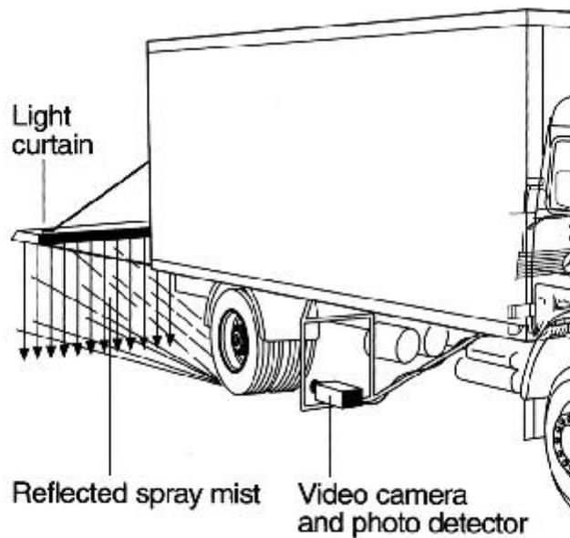
Fig. 9.116 Test setup on commercial vehicle, after H. GÖTZ and R. SCHOCH [9.40].
