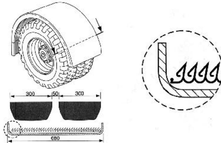
Fig. 9.115 Cross-section of mudguard with grooved section, after H. GÖTZ and R. SCHOCH [9.40].
