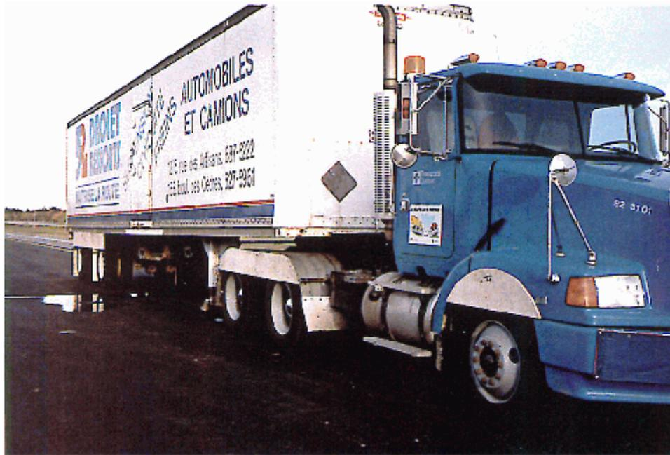
**Figure A-3. Reddaway Side-Valances Mounted on Tractor and Semitrailer (Dumas, Lemay et al. 1998).**
