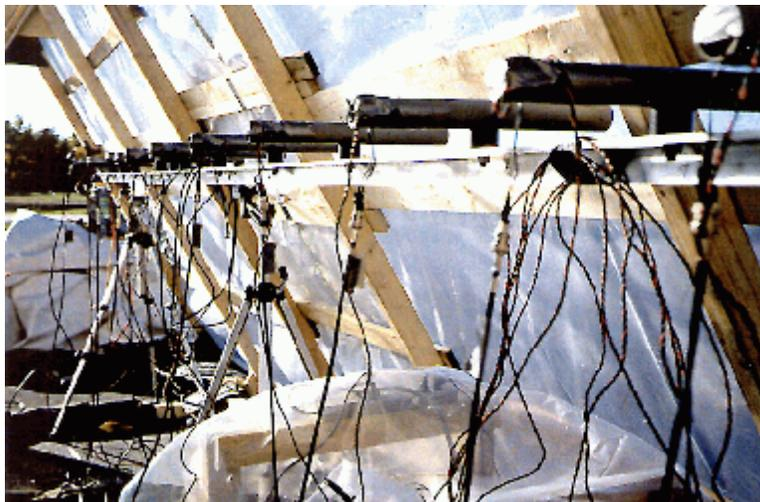
**Figure A-4. Laval University Test Track and Photo-Diodes Used to Measure Spray Intensity (Dumas, Lemay et al. 1998).**
