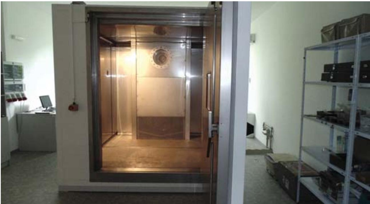
*Fig. 2 Climatic chamber for temperature/humidity tests TCZ 6005 S(m)*
