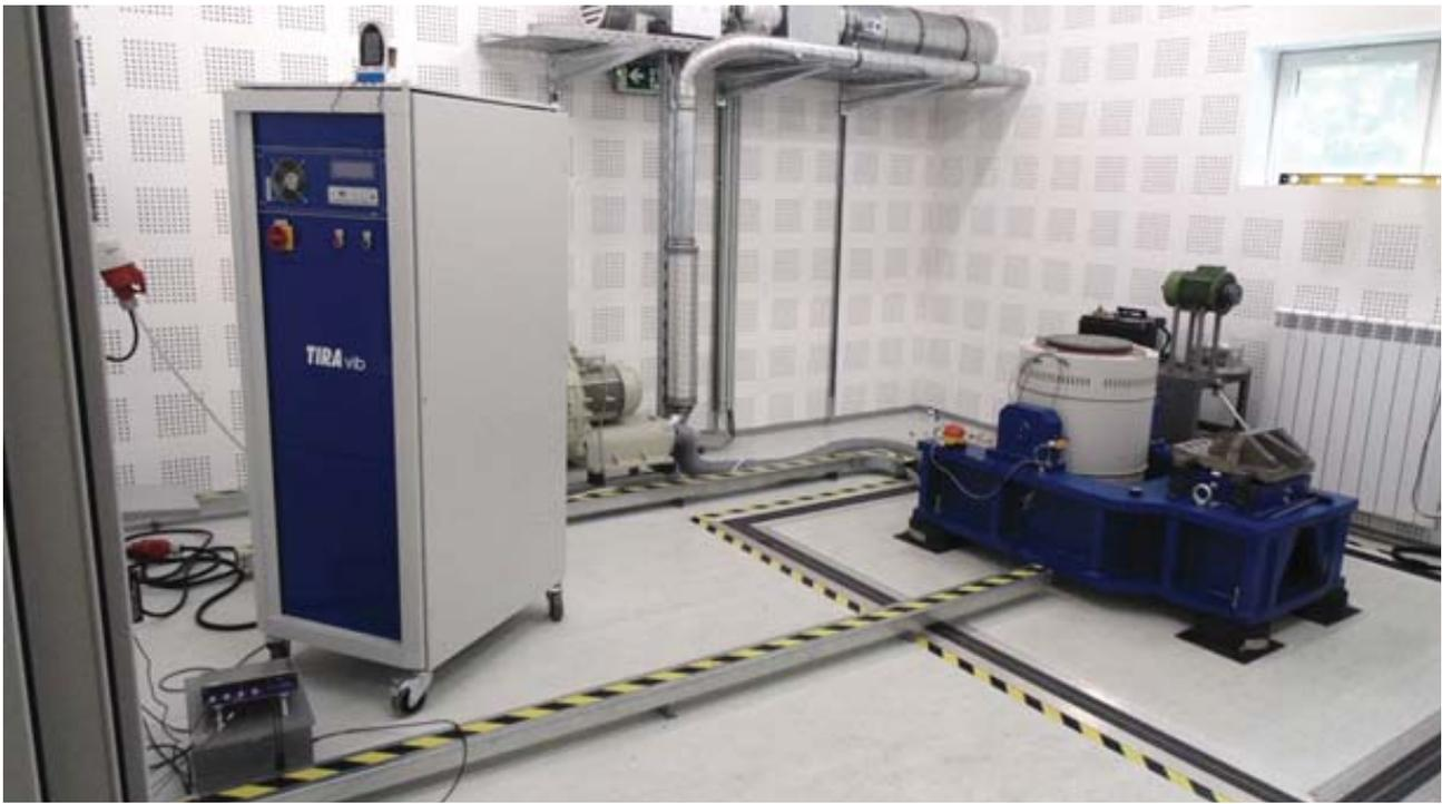
*Fig.1 Vibration test system*
