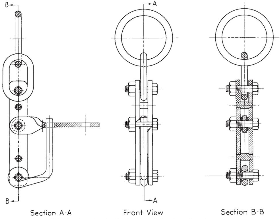
FIG. X1.2 Tripping Device for Hoist-Sling Drop Test Apparatus
