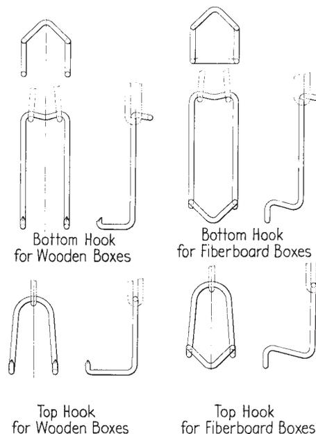
FIG. X1.1 Hooks for Hoist-Sling Drop Test Apparatus
